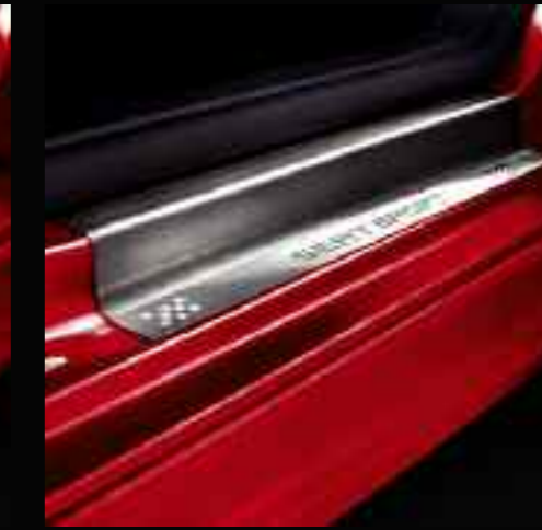
Personalised SEAT Sport sill guards manufactured in stainless steel (6L5071510).
