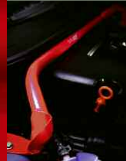
Strut brace made from highly resistant steel (6L0071710).
